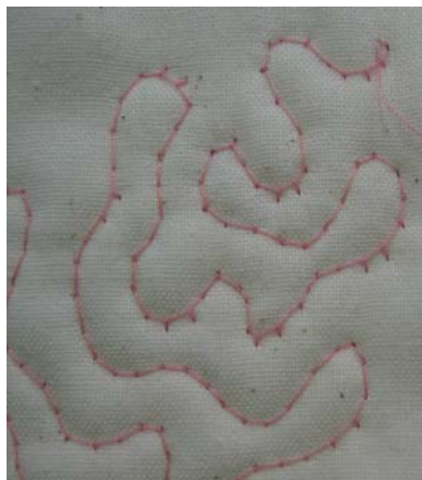
Poor Tension (wrong side)
